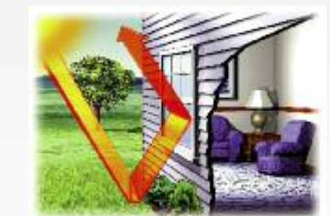
Low-E glass filters long-wave radiation from the sun. This reduces solar heat gain from the summer sun, helping to keep your home cooler.
